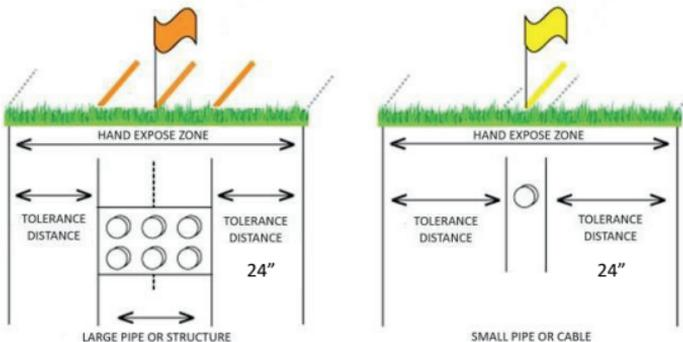
To avoid damaging buried facilities, an excavator shall determine the precise location of underground utilities which have been marked.
