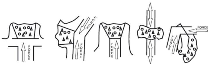
Example: At 25 psi, an 8-inch line could have 1,256 pounds of force exerted on the thrust block. At 200 psi, this 8-inch line could have 10,048 pounds of force exerted on the thrust block. (Not considering surcharging).
