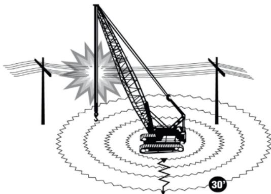
**The equipment operator may try to remove the contact (only if it is safe to attempt)** unaided, and without anyone approaching the equipment. Move away from the line in the reverse direction to that which caused the contact (for example, if you swung left into the wire, swing right to break the contact).
